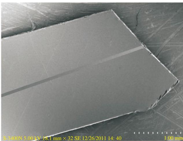
Figure 4. SEM image of patch.
