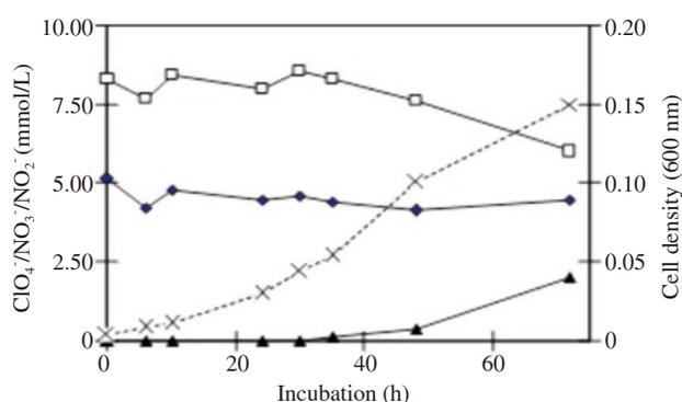
**Figure 3.** Effect of nitrate on perchlorate reduction and growth. ♦: Concentration of perchlorate; □: nitrate; ▲: nitrite; ×: during growth on acetate as indicated by changes in the cell density.
