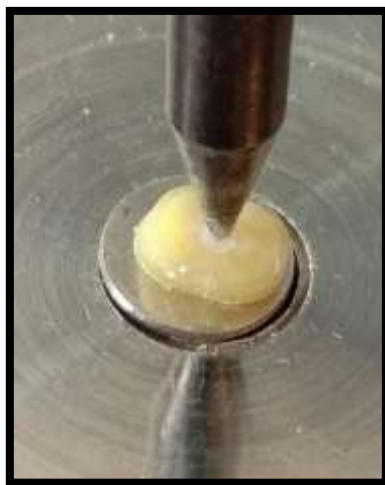
Figure-1: Placement of plunger head for pushout bond test
