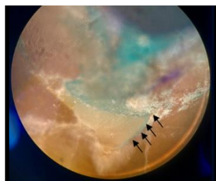
2- dye penetration extending to the inner half of the sealant
